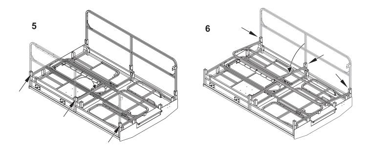
Figure 4-5. Platform Rails - Fold Down Sequence - Main Platform Side Rails
