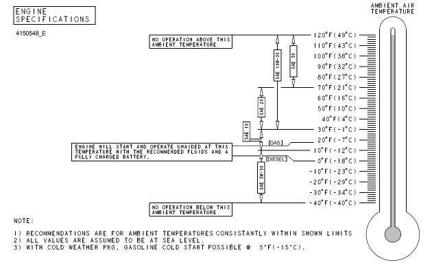
Figure 6-1. Engine Operating Temperature Specifications (Kubota)- Sheet 1 of 2
