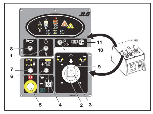
Figure 3-2. Platform - Control Station
