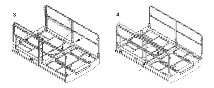
Figure 4-4. Platform Rails - Fold Down Sequence - Deck Extension Side Rails
