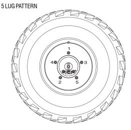
3. The tightening of the nuts should be done in stages. Using the recommended sequence, tighten the nuts per wheel torque chart following.
