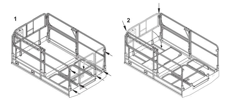
Figure 4-3. Platform Rails - Fold Down Sequence - Front/Rear Rails
